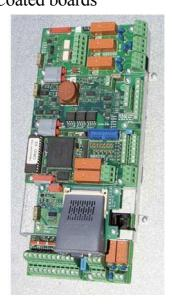
All drive boards are also available as coated, recommended e.g. for sewer pump applications (chlorine gases) or installations with occasional high humidity (if machine room installation or tropical climate). IEC60721-3-3 gases class 3C3, solid particles class 3S2.
