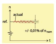
Closed loop = 0.01 % of nnom. Open loop = 0.1 % of nnom. Speed Control dynamic accuracy (impact drop):
