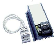
Together with the output choke, the overshoot clamp restricts the voltage and the dV/dt on the motor winding. For rated voltages 380 - 690 V. H x W x D =  $250 \times 145 \times 95 \text{ mm}$
