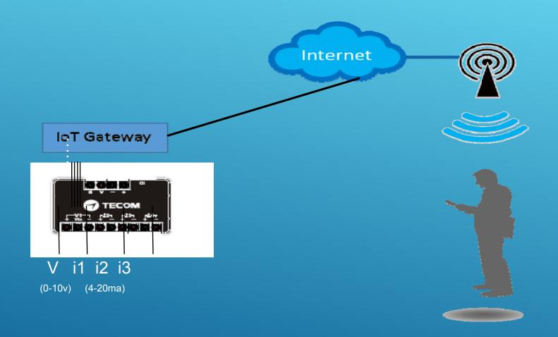
The output from pump Pressure or Flow sensors are accessed via IoT gateway.
